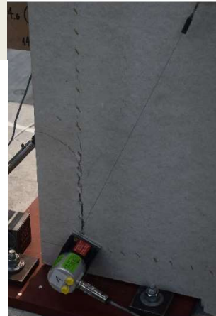
Point A Displacement -25 [mm] IDR = 0.92
