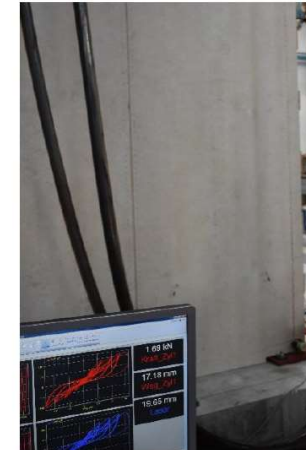
Point B Displacement -30.6 [mm] IDR = 1.13
